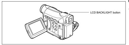
You can switch the brightness of the LCD screen between normal and bright by pressing the LCD BACKLIGHT button. This is useful for outdoor recordings.
